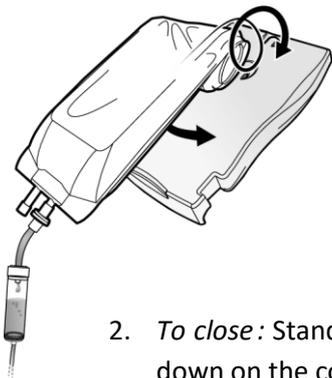
If the bag shape is longer than the plate, fold the bag end on itself in order to meet a length  $\pm$  equivalent to the plate length.
